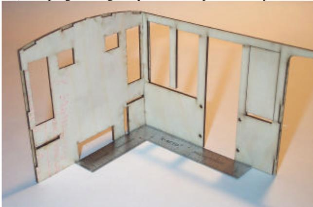
□ Glue the front panel to one side wall, using a square to keep the corners at *exactly* a 90° angle. **Keeping these corners perfectly square is extremely important; take care in this step to insure success later in the rest of the project.** If you do not have a square, use one of the roof panels to check the angle. Make sure that the tabs in the side panel fit snugly into the notches on the front panel. Let dry. □ Repeat with the back panel and the other side wall.
